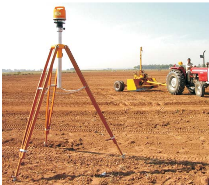
Figure - 7: A View of Agro-Laser based land leveling of agricultural field
